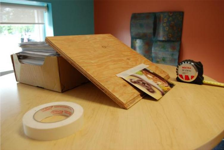
The launch ramp. Ideally, it should be higher and longer. It should also be taped or glued. The cardboard at the base acts as a transition between the ramp and the table to avoid rebounding.
