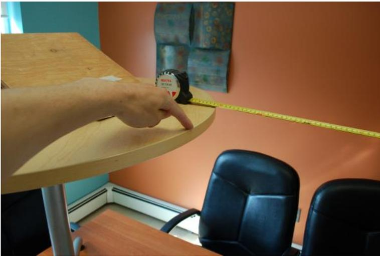
Pointing the origin. That's where the projectile left the table and started free falling.  $F = m * g$  is the only force applied to the projectile, if you don't consider air resistance.
